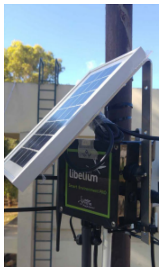
Air quality monitoring solution based on Waspnote Plug & Sense! and Meshlium Gateways
