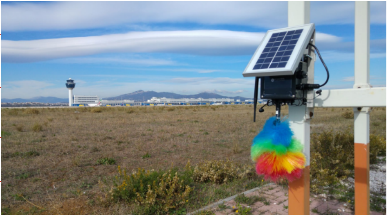
Noise sensors based on Libelium's Waspote Plug & Sense! Smart cities
