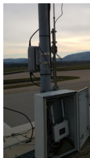
Air quality monitoring solution based on Waspnote Plug & Sense! and Meshlium Gateways
