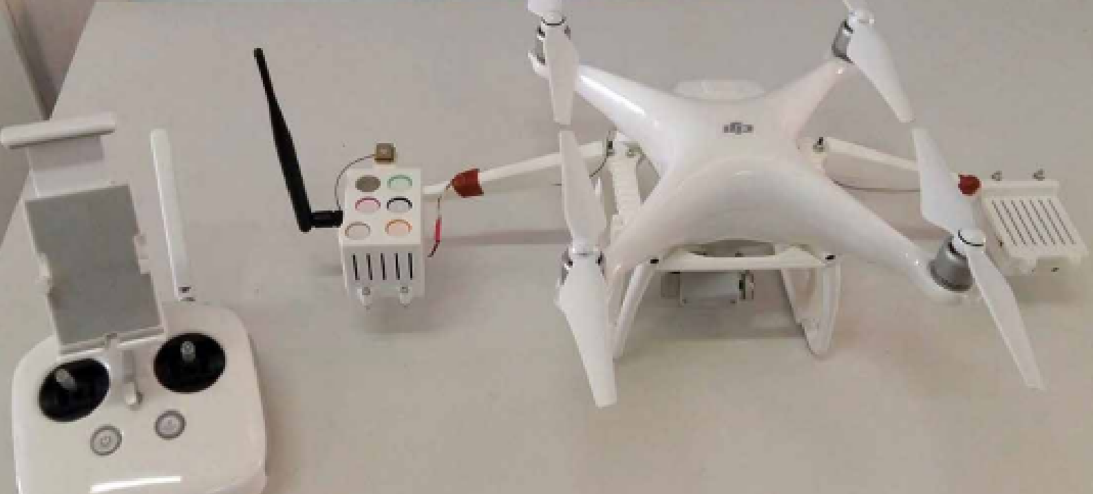
Drone + Calibrated gases wireless sensor platform
