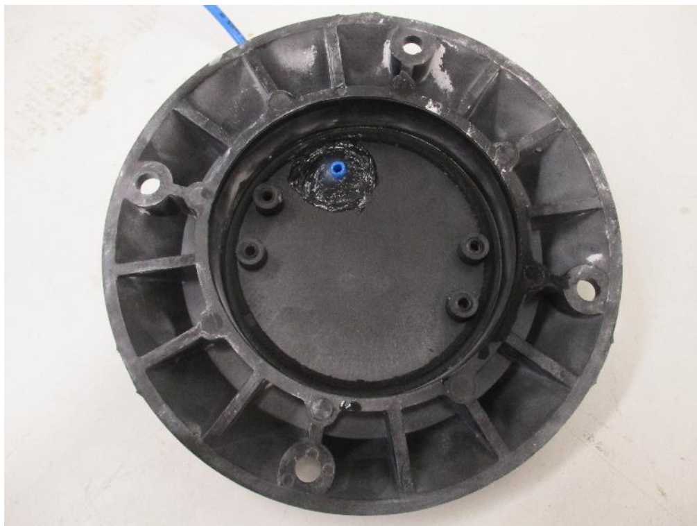
Detail of sample 8061/1 after IP6X test
