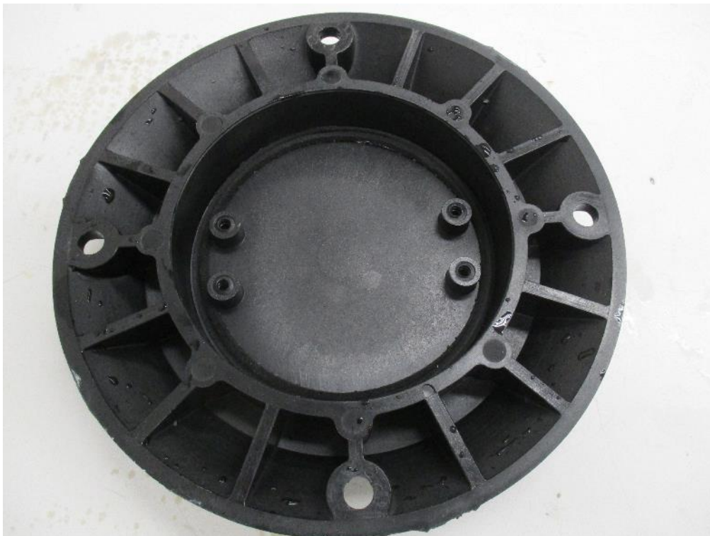
Sample 8061/1 after the IPX8 test
