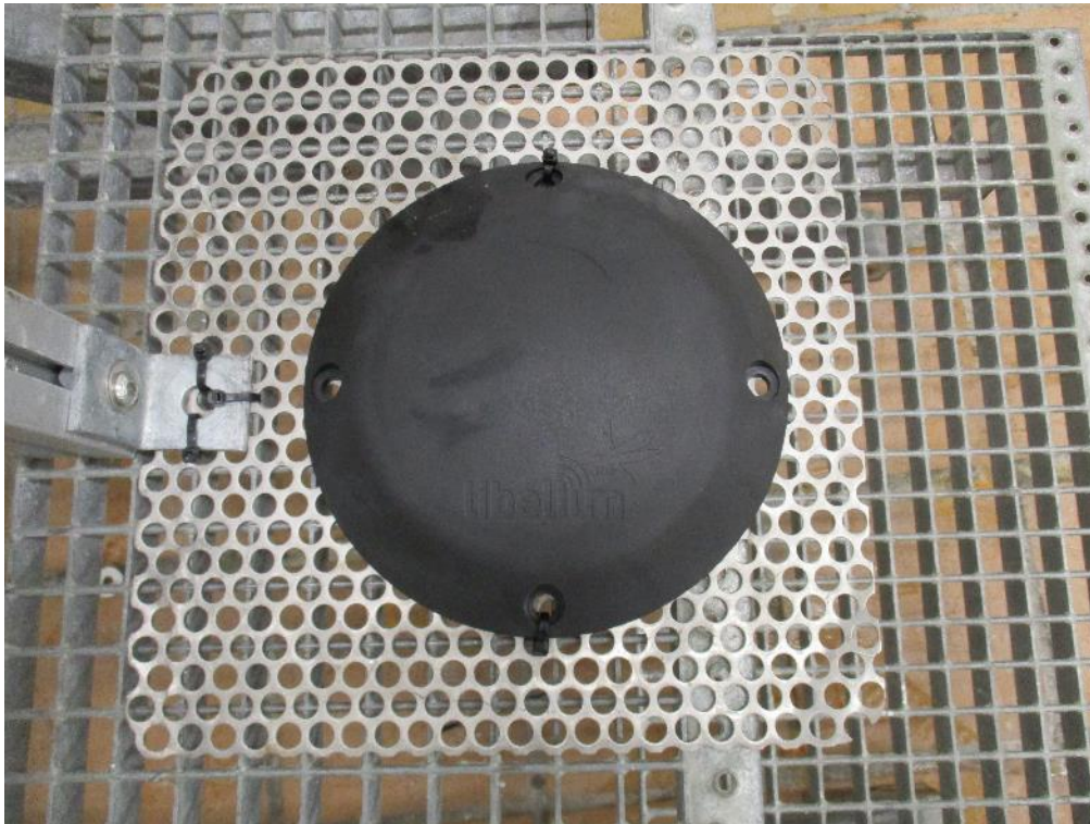
Sample 8061/1 before IPX8 test.
