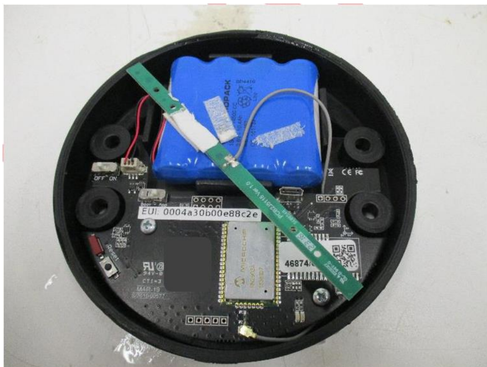
Sample 8061/1 after the IPX8 test
